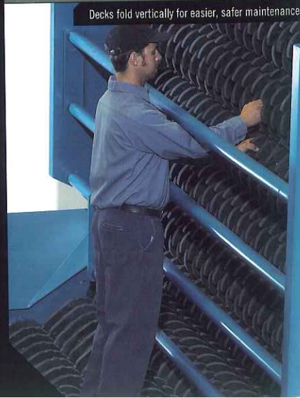
Decks fold vertically for easier, safer maintenance
