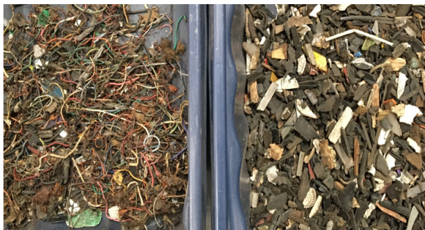
Wire/ICW from ASR/ELV
