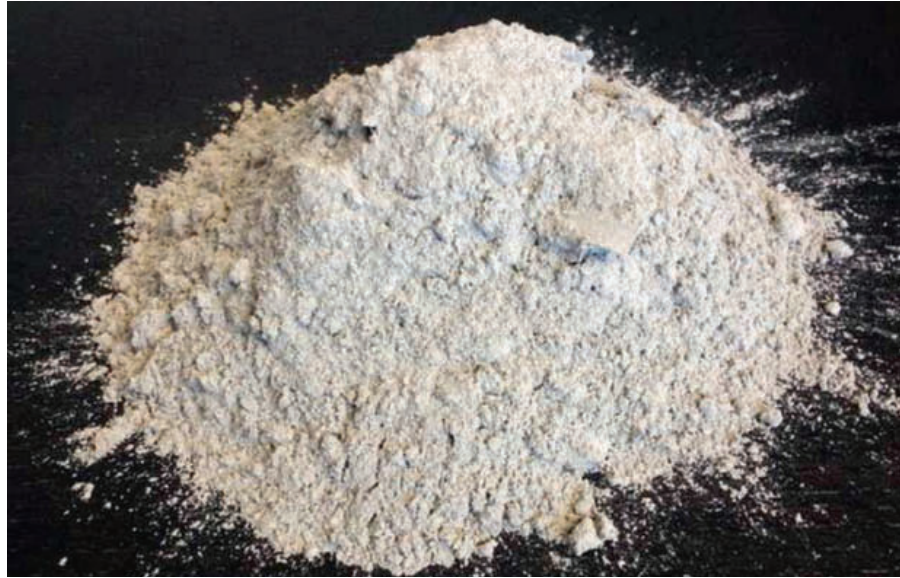
▲ Fluorescent powder containing valuable rare earth elements is vacuumed into special drums
