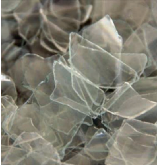
▲ Glass fraction recovered after treating fluorescent lamps in the Blubox unit
