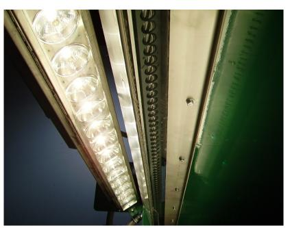
MSS sensors uses only 800 watts per meter of width.
